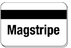
When loading magnetic stripe cards, make sure the stripe is on the left and underneath when viewing from the front of the printer.
