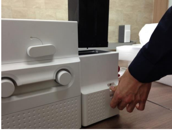
Figure 134 Card jam in Output Hopper 4
