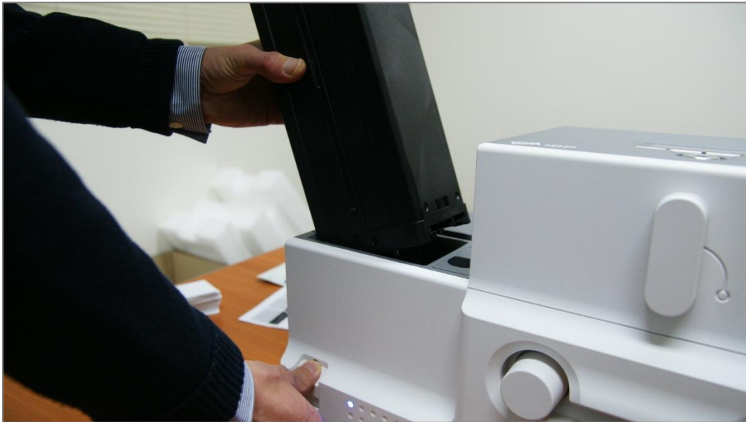
Figure 32 Card cartridge release from Input Hopper
