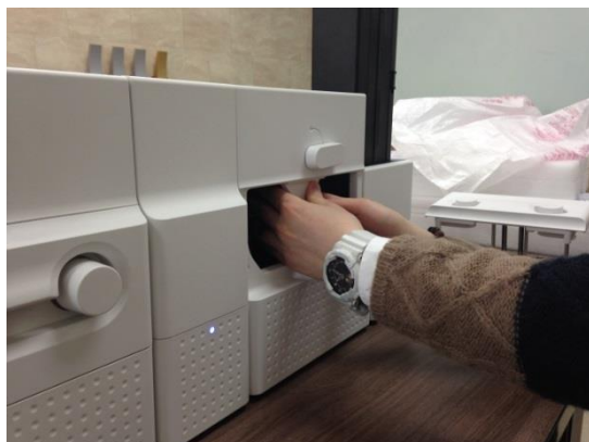
Figure 162 Laminator Head replacement 6
