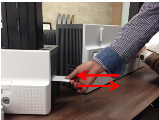
Figure 114 Card jam in Input Hopper 3
