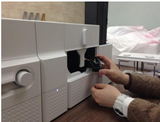
Figure 160 Laminator Head replacement 4
