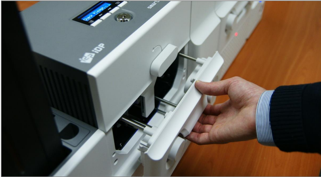
Figure 20 Pulling out ribbon / film cartridge
