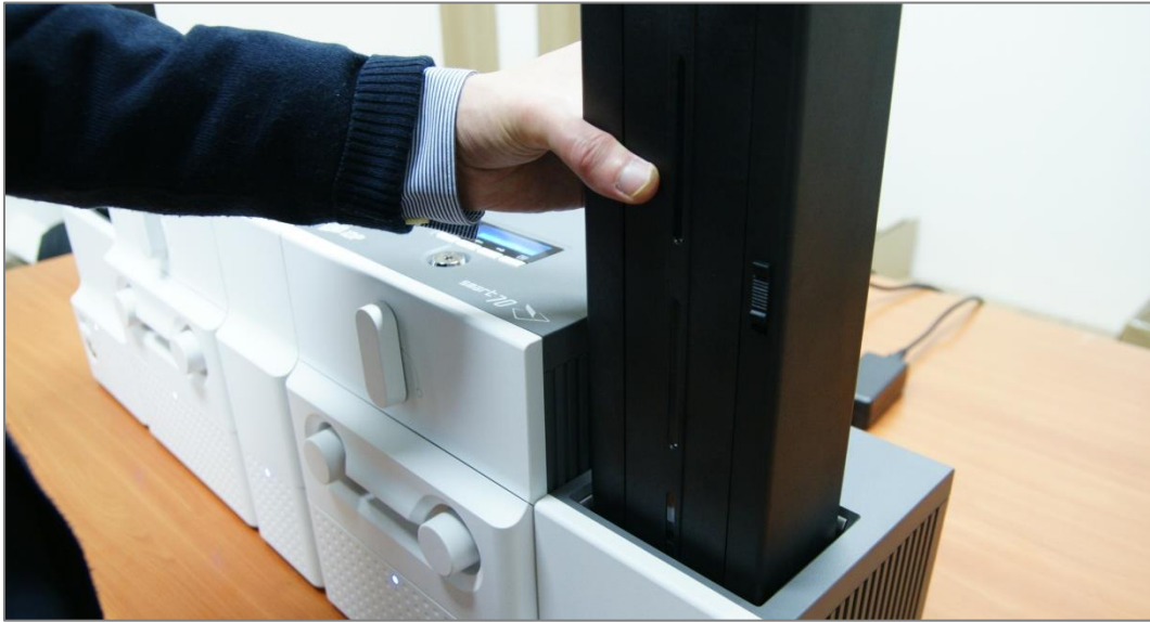
Figure 40 Loading card cartridge into Output Hopper
