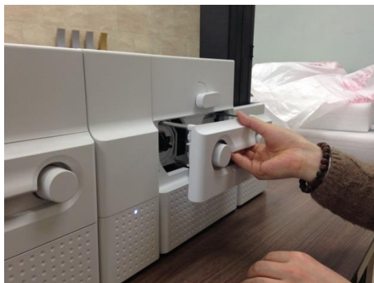
Figure 127 Card jam in Laminator 2
