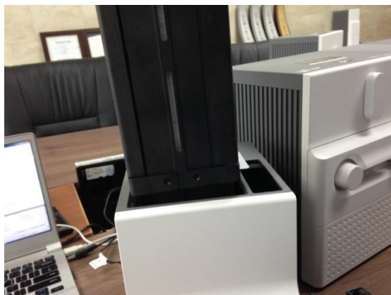
Figure 116 Card jam in Input Hopper 5
