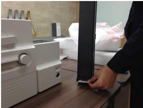
Figure 135 Card jam in Output Hopper 5
