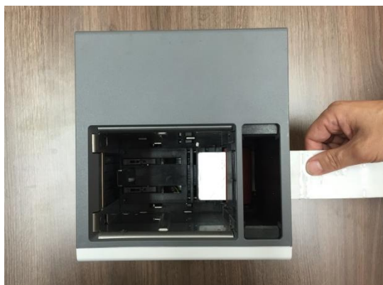
Figure 139 Input Hopper cleaning 4
