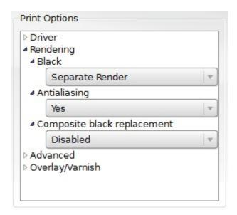
Black - configures how the black color is sent to the printer. You can **Send as RGB**; **Send as Monochrome**; **Send as RGB and Monochrome**; **Send Composite**; **Send Composite and Monochrome** or send as a **Separate Render** (default option).
